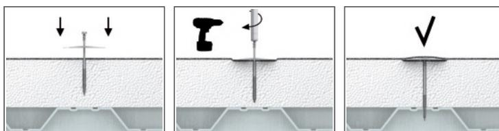
1. Position POW washer on insulation and insert: WBT, WCS, WW screw
